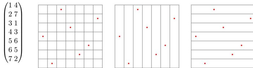
Fig. 1. A Latin Hypercube Design of  $n$  in two dimensions is defined by a permutation of  $n$  symbols. The projections of the design on the coordinate variables are uniformly distributed.
